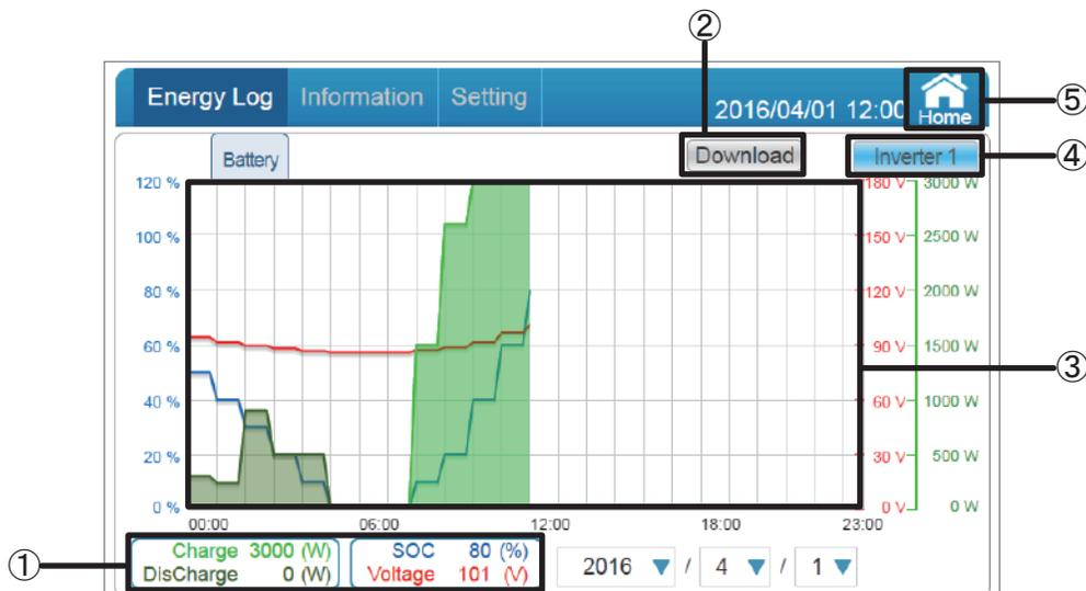
① The details on respective electric power attributes are shown with color coded line graph (Charge: Green/Discharge: Dark Green/SOC: Blue/Voltage: Red).
