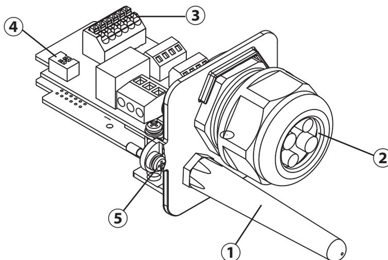
① Wireless Communication Unit Antenna for Inverter
