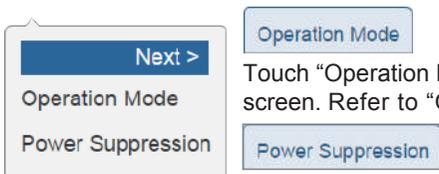
Touch “Operation Mode” to switch the display to the Operation Mode screen. Refer to “Operation Mode” (Page 72) for details.
