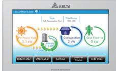
Smart energy monitor to control and optimize the system and the power usage of the owner.
