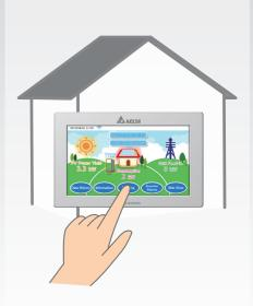
7-inch touch screen monitor provides complete local monitoring without encryption concerns
